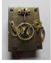
It is "time only" (i.e., no chimes), weight driven, eight day with counter balanced wheel work and a Geneva stop-work mechanism to mechanically stop the winding drum when fully wound to prevent damage from over-winding. The plates are thick brass, which is typical of very high quality clocks. The power of the ten pound weight is controlled by a recoil escapement regulated by a gilded wood pendulum and a zinc bob covered with brass facing.
